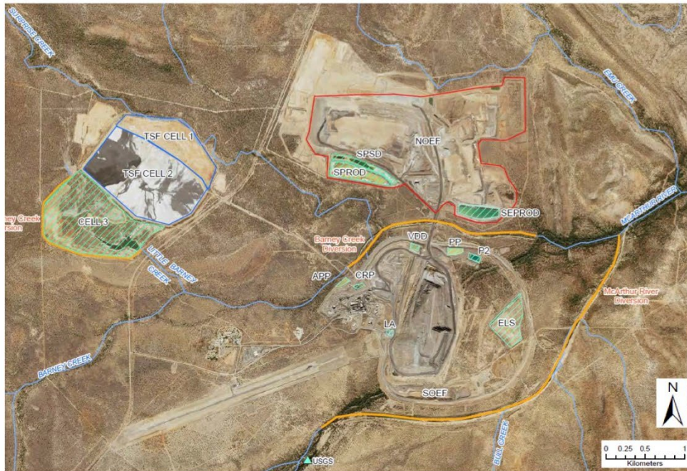
Figure 1: MRM site in 2016 showing the TSF, NOEF, and the open pit. The McArthur River flows towards the north-east, bypassing the open pit via the McArthur River diversion. Barney Creek has been diverted to the north of the open pit, incorporating the flows of Surprise Creek and entering the old channel of the McArthur River before joining with the active McArthur River channel. Source: Ecological Australia (2017)
